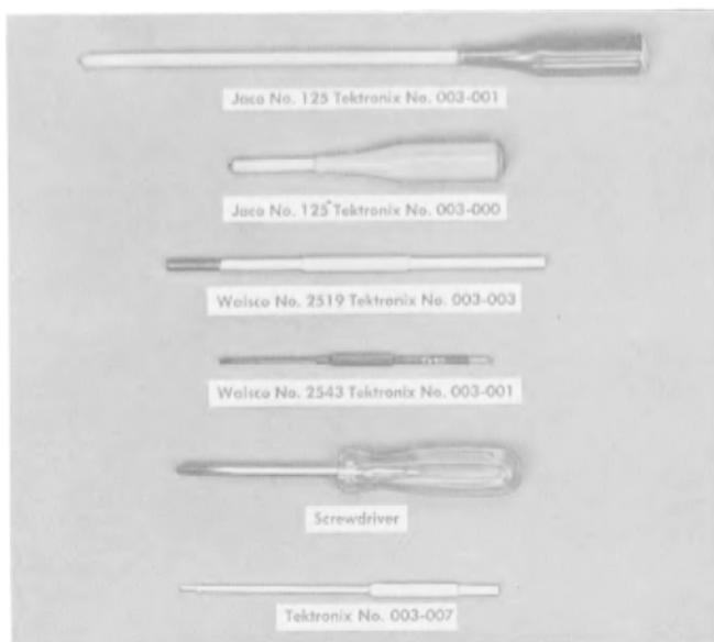
Fig. 2. Calibration tools for use with Type 81.
